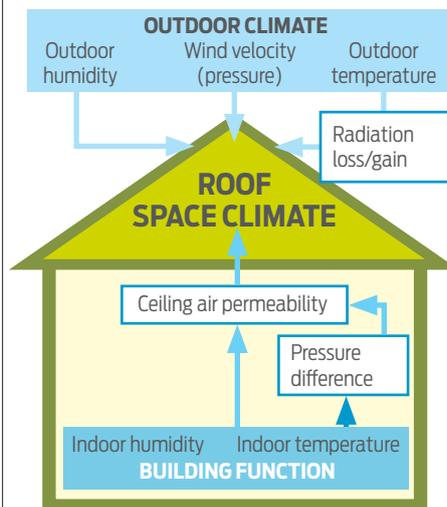
Figure 1: Parameters influencing the roof space climate.
