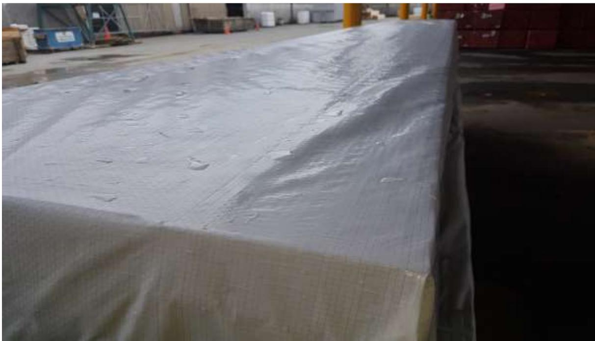
The membrane used for pallet wrapping by the majority is watertight polythene and non-breathable. It is tightly wrapped to top and all side elevations but not the underside. This task is undertaken in the wrapping shed where the stacked timber pallets are generally standing for several weeks depending on current demand. This is the period, especially in the wetter winter months where the moisture content can increase prior to wrapping.
