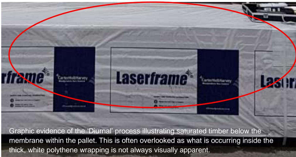
Below: An example of the same problem but here we have clear polythene which visually illustrates the effect polythene has on wrapped timber. This image was actually from another case study showing how the timber was wrapped in the suppliers yard and delivered to site.
