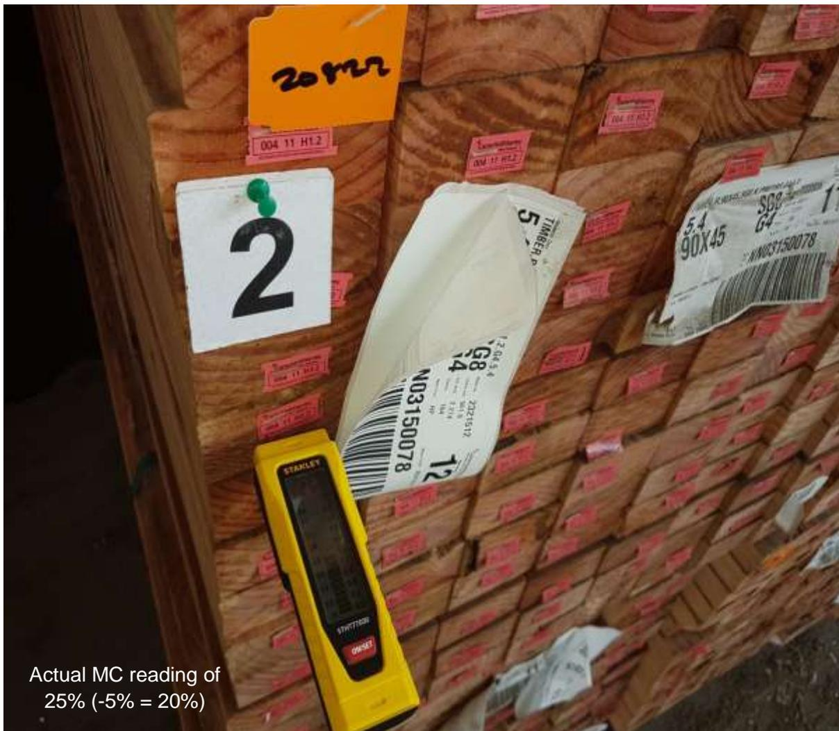
The image above and below illustrates a moisture reading to the end and side of the same piece of timber. It was located centrally within the wrapping shed to the edge of the pallet meaning it would have been generally protected from direct rain but open to RH (Relative Humidity)
