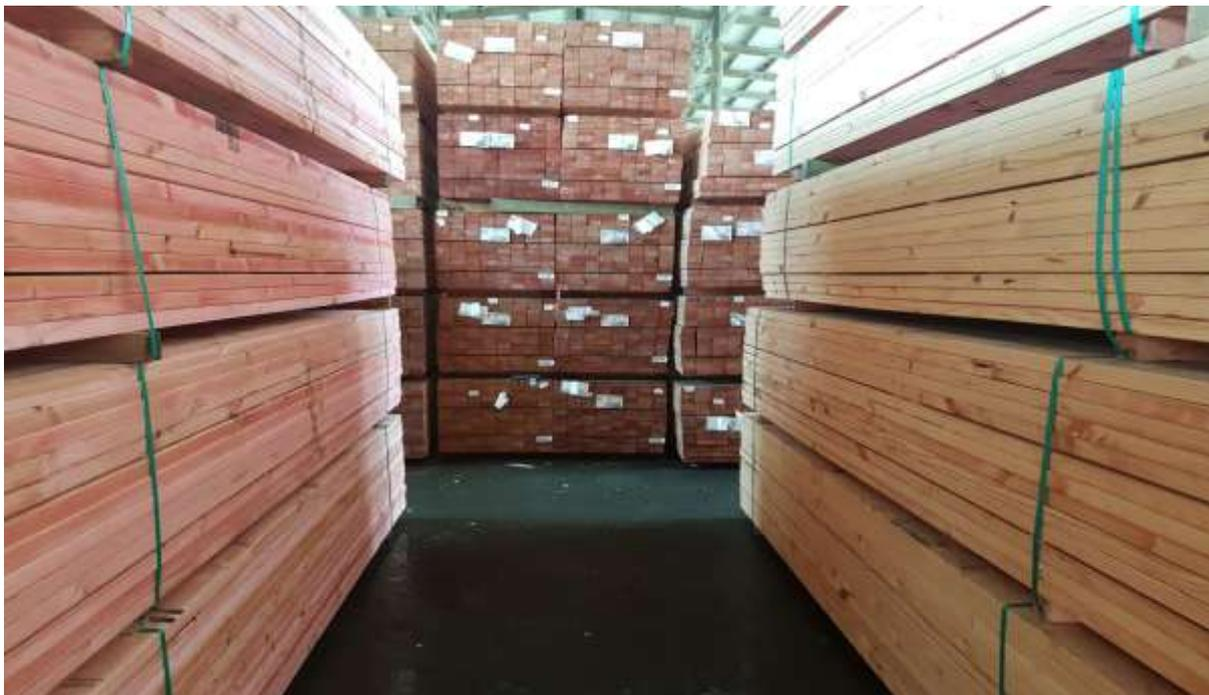
Above: Tightly stacked timber with reduced airflow to centre of shed location also illustrating the volume of moisture on the concrete floor slab. Relative Humidity averaging 70%.
